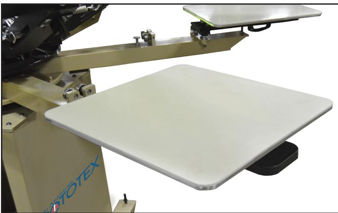
Durable quick-release aluminum pallets are heat-resistant and warp-proof.
